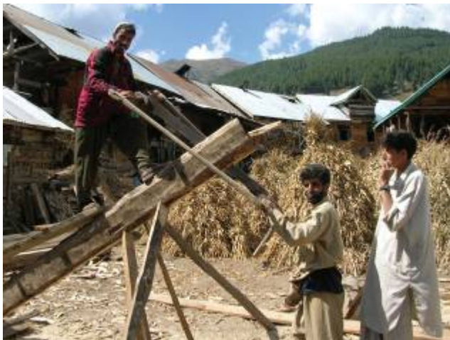
Figure 4&5: Left: Hand sawing of log into boards, 2006, a still common practice in rural Kashmir, India. Photo by ©Abbid Hussain Khan for INTACH. Right: Balloon frame house washed downstream but remained intact when dam burst in Jonestown, Pennsylvania, 1889 killing 2209 people.
