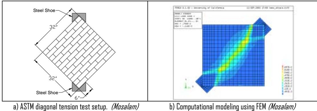
**Figure 4: Proposed test setup and accompanied computational modeling**
