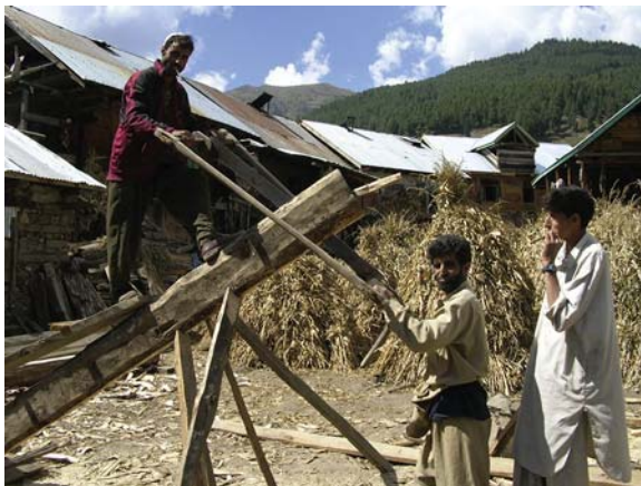
Figure 1.15 Contemporary continuation of preindustrial technique of sawing timbers into boards in Kashmir.
